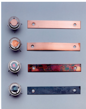
Figure 1: Environmental reactivity coupons (ERCs) showing corrosion.
